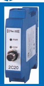
The 2C20 Module provides electrical interface to the Allen-Bradley ControlNet protocol by conditioning the electrical signals supplied to and from the ControlNet network for transmission over fiber optic cable.
